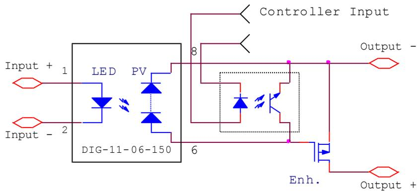
**5. Open Thermocouple Detector:**
