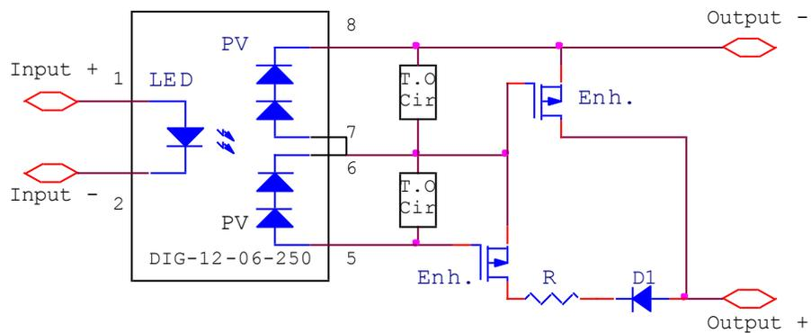
**4. Power MOSFET Photovoltaic SPST N/O Relays With Opto-Transistor for High Speed Turn-Off:**
